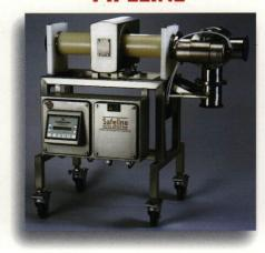
Pipeline systems inspect pumped liquids, paste and slurry such as meat emulsion, cheese, peanut butter, soup and sauces in a wide range of temperatures and pressures.
